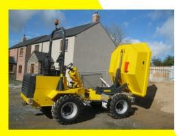
2 speed Hydrostatic Drive providing superb climbing ability.
